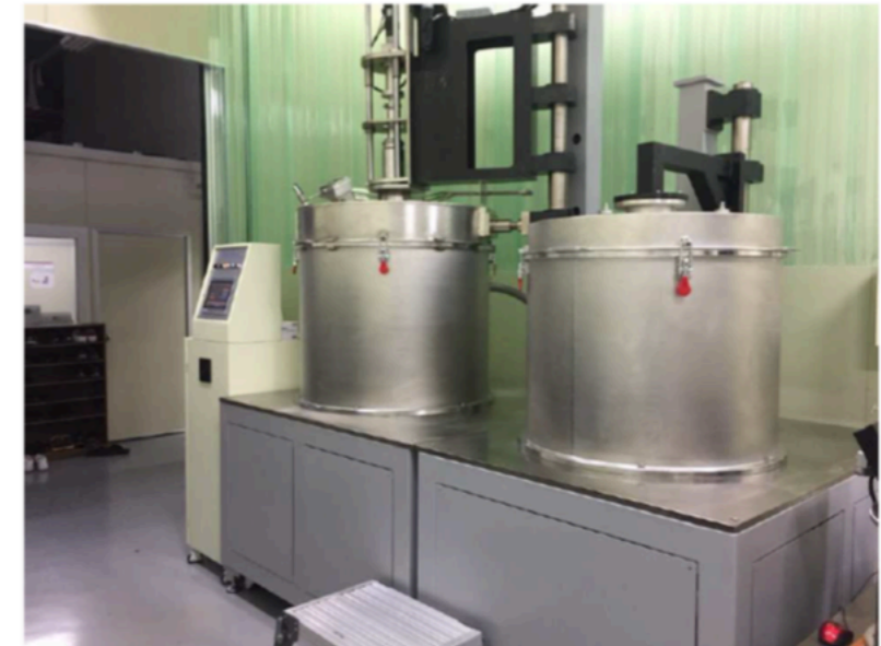
~ 100 kg NaI crystal (ingot) grower
